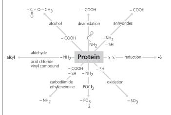
**Figure 2.2** The numerous and diverse side chains of proteins offers the polymer scientist limitless opportunities to specifically tailor the properties of the final polymeric material by using chemical modification.
