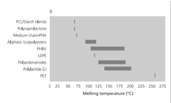
**Figure 2.5** Comparison of the thermal properties of biobased polymers with conventional polymers. (All data is from company information).
