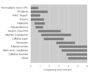
**Figure 2.6.** Indication of the time required for composting of various biobased and synthetic polymeric materials. Measurements of composting times were performed at ATO. The durations presented in this figure are based on an intermediate level of technology as observed in actively aerated and mechanically turned hall composting.
