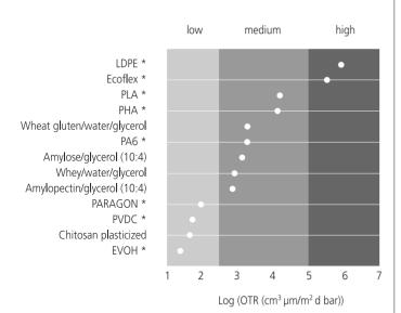
**Figure 2.3** Comparison of oxygen permeability of biobased materials compared to conventional mineral-oil-based materials. Permeability of materials marked with \* was measured by ATO, Wageningen, NL (23°C, 50% RH), information on other materials is based on literature (Rindlav-Westling et al., 1998; Butler et al., 1996).
